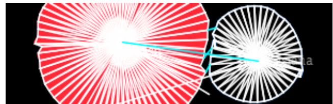
Figure 2 Detail of the springs responsible for the system's behavior. The white lines represent the springs that form each body skeleton, as well as the per body geographic attractor. The temporary springs that implement bodies' collisions are represented in cyan.
